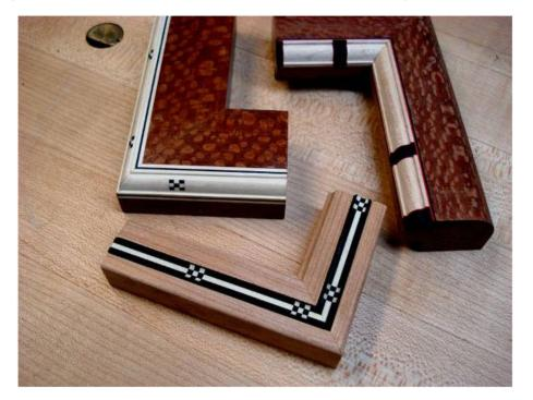
Rutager starts by re-sawing solid stock and running it through a Performax sander to get very thin wood. He laminates these thin strips together to make multi-colored sandwiches that he uses to make the inlays.
