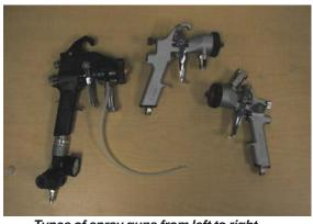
Types of spray guns from left to right pressure, siphons, and gravity feed
