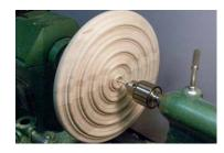
8. Turn beads and coves. Finish sand and seal front face. Drill small pilot hole through the disk, to mark center. Pry piece from drive facepleate with wood chisel.
