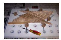
16. Groups of 4 re difficult to clamp. A fixture such as this aids in holding irregular shapes. Following glue-up, sand rear face flat, and finish with spray finish.
