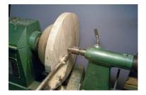
3. Trap blank between faceplate and tail stock with firm tail stock pressure. Start lathe slowly and assure blank is secure.
