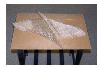
14. Glue fragements together two by two, with PVA glue. Use water, brush, and rag to clean any excess glue from face. Clamp time as recommended on glue bottle.
