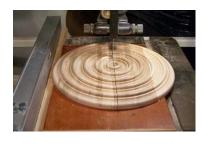
9. Make carrier board, guided by band saw fence. Cut turned piece on center along wood grain. Sand cut edges and make each half equal in size.
