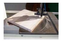
1. Cut 12" diameter disk from four quarters rough cut material with band saw. Pictured is soft maple.
