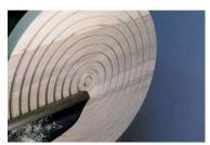
7. Layout alternating 3/8" wide beads and coves separated by 1/8" wide fillets. Cut fillets 3/16" deep.
