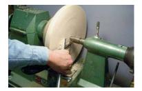
4. True-up one side of blank. Sand off small nubbin where blank is held by the tail stock. Reverse and true-up other side.
